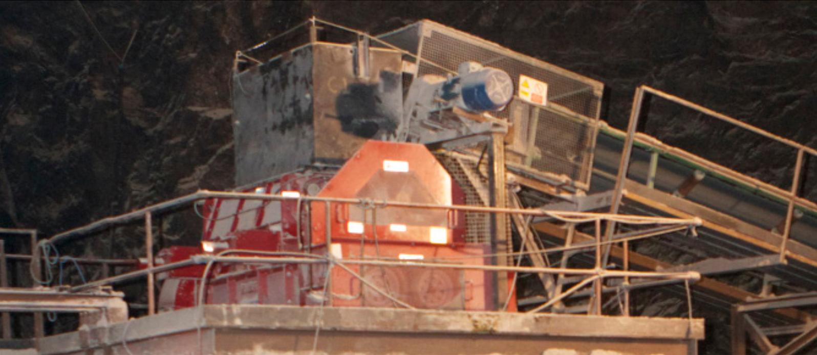
Triple Roll Crushers allow producers to accomplish two stages of reduction in a single crusher. Multiple duty classes are designed for use in coal, salt, coke, glass, trona, and other mineral processing applications. Triple Roll Crushers are capable of achieving a 6:1 reduction ratio in the primary crushing stage and a 4:1 reduction ratio in the secondary stage. This two-stage crushing system produces a cubical product at a high capacity.
