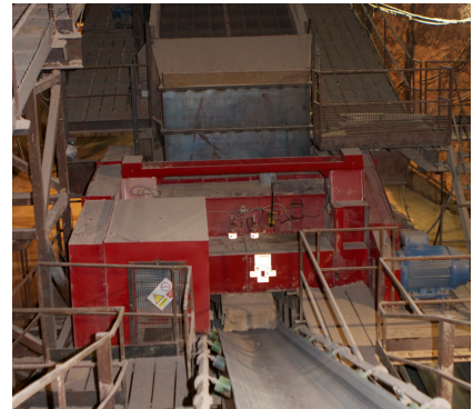
Double Roll Crushers can be installed above or underground.
