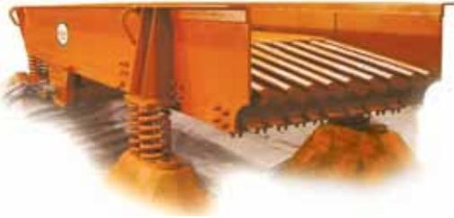
The Universal Vibrating Grizzly Feeder provides a continuous feed rate under a variety of loading and material conditions. Rugged construction takes the heavy shock loads of trucks, shovels and loaders. The main frame is comprised of deep fabricated side frames and heavy-duty cross-members, all welded and stress-relieved into a unit which gives you years of maintenance free service.
